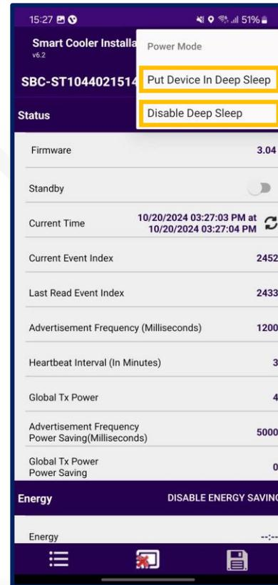
**A. To Disable Deep Sleep** - To disable deep sleep mode, the user must keep the door magnet close to the device then the device starts advertising for 30 seconds. user must connect within 30 seconds to a smart device, Tap on Smart Device and After the connection, go to **Menu > “Power Mode” > “Disable Deep Sleep”**.
